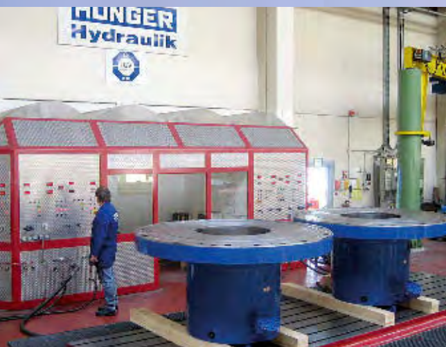
Hydroforming press with four pressing cylinders (Photo and sketch: University of Stuttgart, Institute for Forming Technology)
