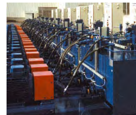
The modern drives have hydraulic control and safety blocks, mechanical and electronic position measuring systems and automatic locking devices.
