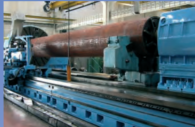
Turning of large parts, dimensions of up to 4 m in diameter and 25 m in length
