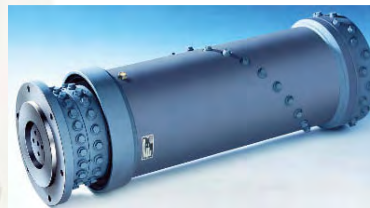
Special rotary transmission with 44 channels for a 4-station special machine with an operating pressure of 300 bar (medium: hydraulic oil)
