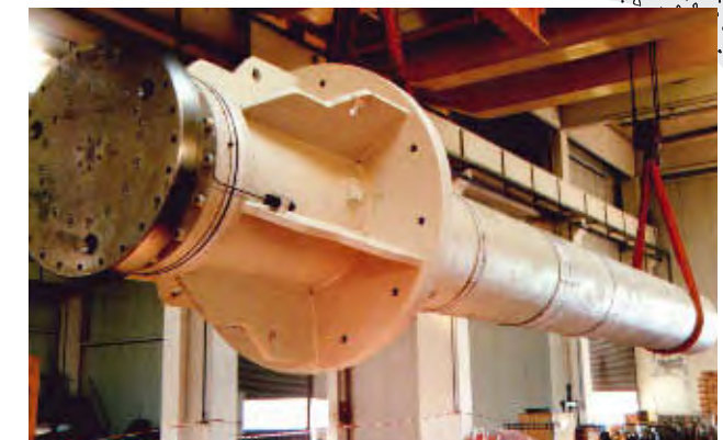
Vertical casting cylinder for aluminum continuous casting Shown schematically on the right when installed
