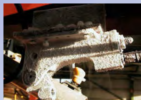
Locking hook for landing gear at a low temperature of -54°C
